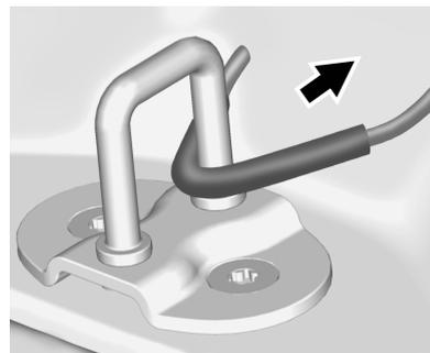
9. Make sure the metal tube is centered at the striker. Push the tube toward the front of the vehicle.
