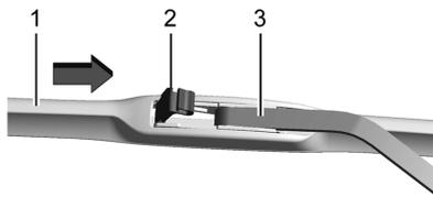
3. With the latch (2) open, pull the wiper blade (1) assembly down toward the windshield far enough to release it from the J-hooked end of the wiper arm (3).
