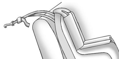
If the position you are using does not have a head restraint and you are using a dual tether, route the tether over the seatback.
