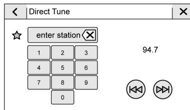
Access Direct Tune by touching the Tune icon on the infotainment display to bring up the keypad. Navigate through all frequencies using the arrows on the right side of the Direct Tune display. Directly enter a station using the keypad. When a new station is entered, the information about that station displays on the right side. This information will update with each new valid frequency. Touch to save the station as a favorite.
