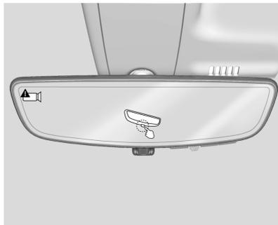
See your dealer for service if a blue screen and
