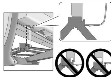
5. Turn the wheel wrench clockwise to raise the jack lift head until the slots in the jack head fit into the metal flange behind the contact with the plastic molding. Do not raise the vehicle yet.
