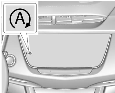
The automatic engine Stop/Start feature can be disabled and enabled by touching the (A) symbol. Auto Stop is enabled each time you start the vehicle.
