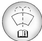
Open the cap with the washer symbol on it. Add washer fluid until the tank is full. See *Engine Compartment Overview* ⇨ 290 for reservoir location.
