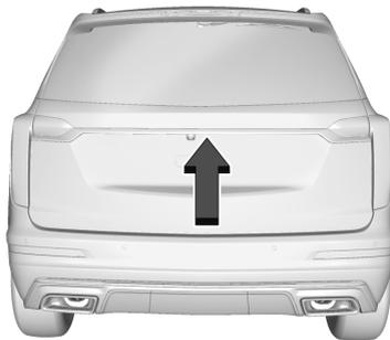
To open the liftgate, press the touch pad under the liftgate handle and lift up.
