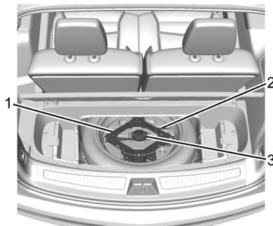
4. Turn the wing nut (3) counterclockwise to remove the jack (1) and wheel wrench (2). Place the tool container near the tire being changed.
