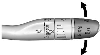
The rear window wiper/washer controls are on the end of the windshield wiper lever.
