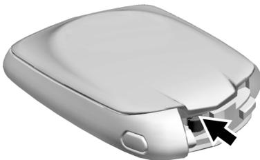
2. Separate the two halves of the transmitter using a flat tool inserted into the bottom center of the transmitter. Do not use the key slot.
