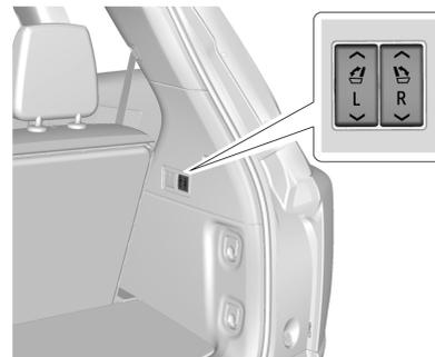
4. To fold the third row seatback from the cargo area, press and hold the seatback folding switch on the passenger side of the rear cargo area.
