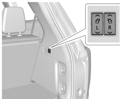
2. To return the seatback to the seating position from the cargo area, press and hold the seatback folding switch on the passenger side of the rear cargo area.
