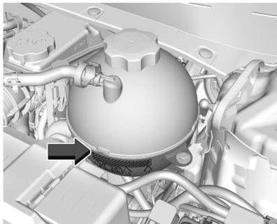
3. Fill the coolant surge tank with the proper mixture to the mark pointed to on the front of the coolant surge tank.
