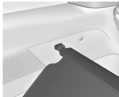
6. Place one of the forward cargo cover ends into the slot and then compress to fit the other end into the corresponding slot in the opposite panel.
