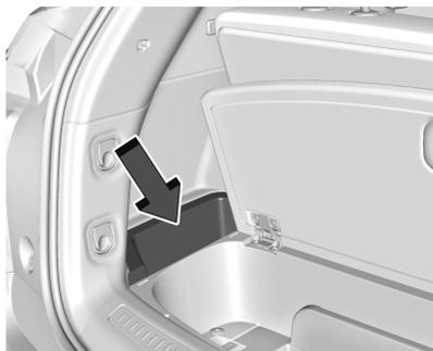
The rear compartment fuse block is in the cargo area, on the driver side of the vehicle behind the lower trim panel. To access the fuses in the Rear Electrical Center, remove the fuses in the Rear Electrical Center, remove the center cargo bin, then small side bin. See *Rear Storage* ⇨ 90. See your dealer if additional assistance is needed.
