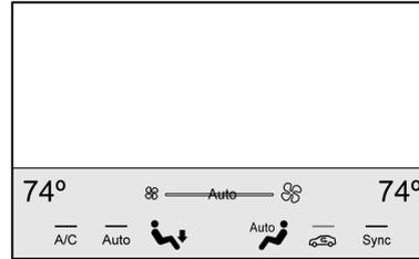
The climate control status display appears briefly when the climate control buttons on the center stack are adjusted. The air delivery mode can be adjusted on the climate control status display.
