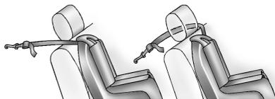
If the position you are using has a fixed headrest or head restraint and you are using a single tether, route the tether around the inboard or outboard side of the headrest or head restraint.
