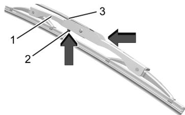
4. Push the release lever (2) to disengage the wiper arm (3) hook from the wiper blade (1) assembly.
