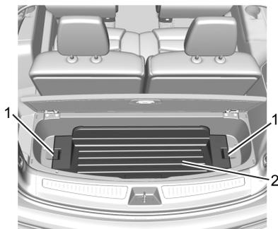
3. Remove the cargo management system tray (2) by pulling on the handles (1). See *Cargo Management System* ⇨ 94.
