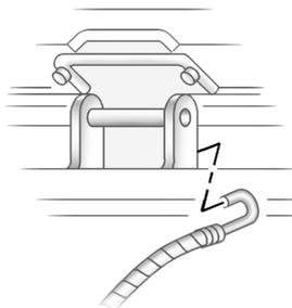
6. Open the lift gate to 3 / 4 door location and adjust the door automatically or manually until there is enough space to hook the cable to the door hinges. See *Liftgate* ⇨ 18.
