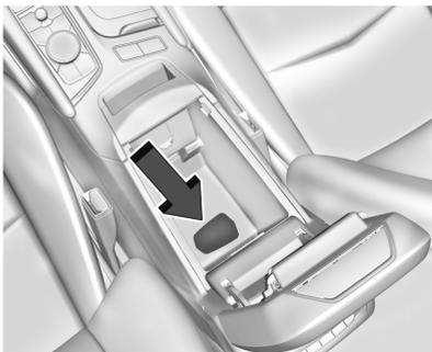
2. Place the transmitter in the transmitter pocket.
