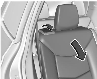
2. Pull the handle on the top of the seat forward and pull the seat forward.
