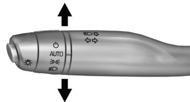
Move the lever all the way up or down to signal a turn.
