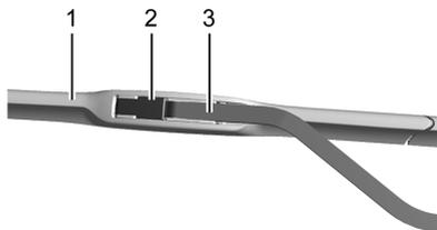
2. Lift up on the latch (2) in the middle of the wiper blade (1) assembly where the wiper arm (3) attaches.
