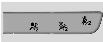
The symbols for on and off will be visible during the system check. When the system check is complete, either the symbol for on or of will be visible. See *Passenger Airbag Status Indicator* ⇨ 113.
