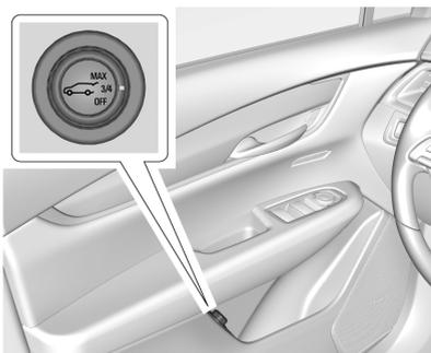
The power liftgate switch is on the driver door. The vehicle must be in P (Park).
