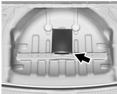
1. Remove the cable package from under the spare tire, jack, and tools.
