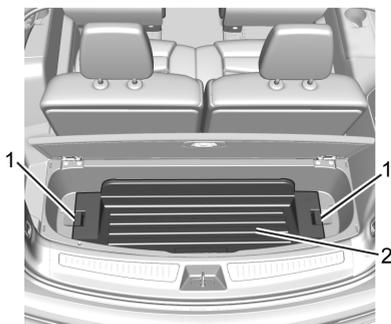
Remove the cargo management system tray (2) by pulling on the handles (1).
