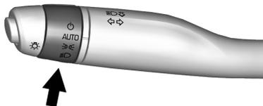
To enable the IntelliBeam system, press the end of the turn signal lever when it is dark outside and the exterior lamp control is in AUTO or
