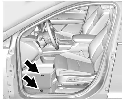
1. Pull up on the rear of the driver side floor mat to unlock each retainer and remove.
