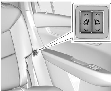
3. To fold the third row seatback from the second row seating area, press and hold the seatback folding switch on the right or left side of the second row seating area.
