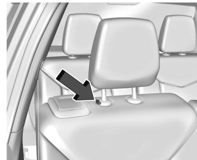
To lower the head restraint, press the button, located on the top of the seatback, and push the head restraint
