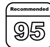
Unleaded petrol with a posted octane rating of 95 RON or greater and with ethanol up to 10% by volume is recommended. If unavailable, unleaded petrol rated at 91 RON can be used, but will result in reduced performance and driveability, and an audible knocking noise may be heard.
