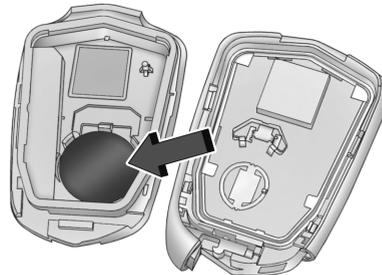
3. Remove the old battery. Do not use a metal object.
