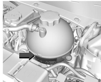
1. With a cold system, disconnect the vent line from the port near the cap on the surge tank. Add coolant to the indicated mark on the surge tank.
