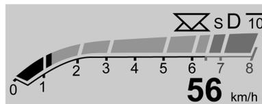
**Performance View :** This displays digital speed, indicators from speed view along with rpm reading, transmission positions, and gear shift indicator (if equipped).
