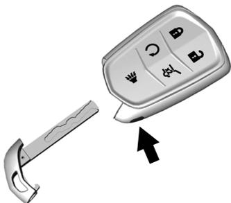
1. Press the button on the side of the RKE transmitter near the bottom and pull the key out. Never pull the key out without pressing the button.
