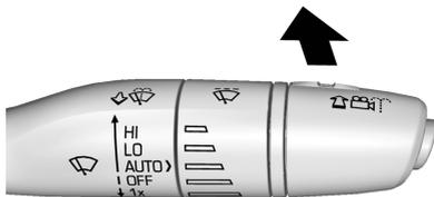
If equipped, push the windshield wiper lever forward to spray washer fluid on the rear camera lens. The lever returns to its starting position when released. See *Rear Camera Mirror* ⇨ 30.
