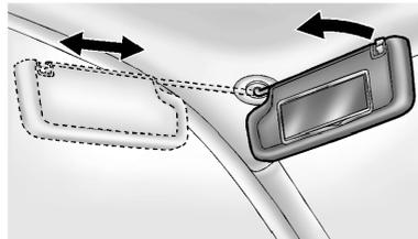
Pull the sun visor down to block glare. Detach the sun visor from the center mount to pivot to the side window and, if equipped, extend along the rod.
