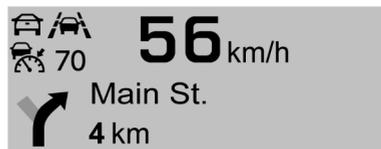
**Navigation View :** This displays digital speed, indicators from speed view along with Turn-by-Turn Navigation information in some vehicles. The compass heading is displayed when navigation routing is not active.
