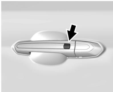
If equipped, the RKE transmitter must be within 1 m (3 ft) of the liftgate or door being opened.
