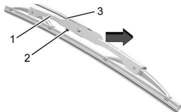
6. Push the new wiper blade (1) assembly securely on the wiper arm (3) until the release lever (2) clicks into place.
