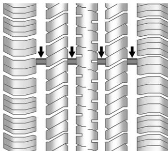
Treadwear indicators are one way to tell when it is time for new tires. Treadwear indicators appear when the tires have only 1.6 mm (1/16 in) or less of tread remaining. See *Tire Inspection* ⇨ 328 and *Tire Rotation* ⇨ 329 for additional information.
