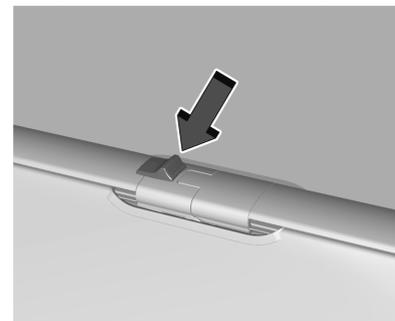
2. Slide the rear crossbar release button and allow the crossbar to fold while lifting. Be sure to avoid finger pinching points as the cover folds.
