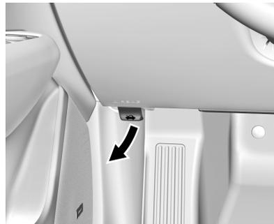
1. Pull the hood release lever with the
