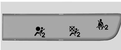
When the vehicle is started, the passenger airbag status indicator will light the symbols for on and off for several seconds as a system check. Then, after several more seconds, the status indicator will light the on or off symbol to let you know the status of the front outboard passenger frontal airbag.
