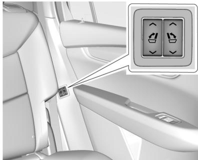
1. To return the seatback to the seating position from the second row seating area, press and hold the seatback folding switch on the right or left side of the second row seating area.
