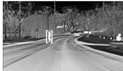
With the Front Pedestrian Braking system turned on, Night Vision provides a red Head-Up Display (HUD) alert when the system detects that the vehicle is approaching a pedestrian ahead too quickly. In addition, an alert beeps or the Safety Alert Seat pulses, if equipped. See *Front Pedestrian Braking (FPB) System* ⇨ 263.
