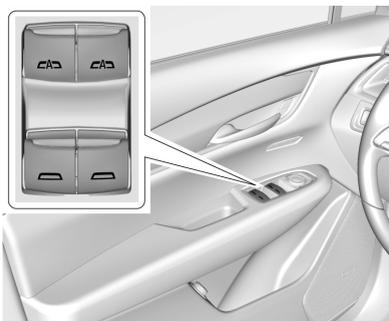
The power windows work when the ignition is on, in ACC/ACCESSORY, or when Retained Accessory Power (RAP) is active. See *Retained Accessory Power (RAP)* ⇨ 222.
