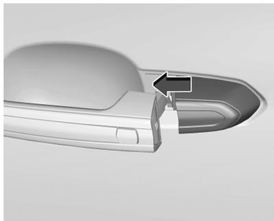
3. Slide the cap forward and press the forward edge to install the cap in place.
