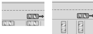
After completely passing an eligible parking spot, a beep sounds and a red stop symbol is displayed in the driver information center. Generally, APA selects the nearest empty parking spot behind the vehicle, but under some conditions may select a space that is further back. Slow down and bring the vehicle to a complete stop to begin.
