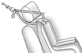
If the position you are using has a fixed or an adjustable head restraint and you are using a dual tether, route the tether around the head restraint.
