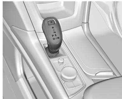
The shift pattern is displayed in the top of the shift lever. The selected gear position will illuminate red on the shift lever, while all others will be displayed in white. If the shift is not immediate, as in very cold conditions, the indicator on the shift lever may flash until it is fully engaged.
