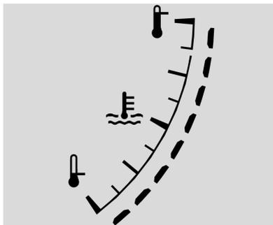
This gauge measures the engine coolant temperature.
