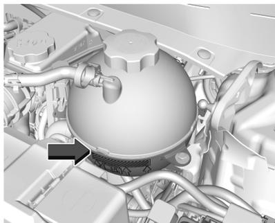
Check to see if coolant is visible in the coolant surge tank. If the coolant inside the coolant surge tank is boiling, do not do anything else until it cools down. If coolant is visible but the coolant level mark is not at or above the indicated mark, add a 50/50 mixture of clean, drinkable water and DEX-COOL coolant. Be sure the cooling system is cool before this is done. See *Engine Overheating* ⇨ 302.
