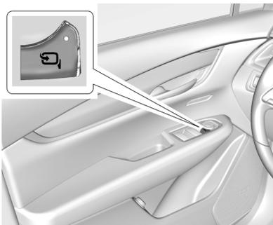
If equipped, press
