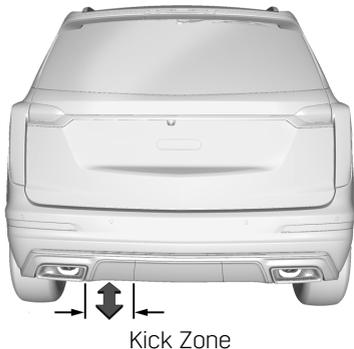
To operate, move your foot in a forward kicking motion under the left side of the rear bumper, at the location of the projected logo, then pull it back. Then step back. The kick must come within 14 cm (6 in) of the rear bumper to activate.
