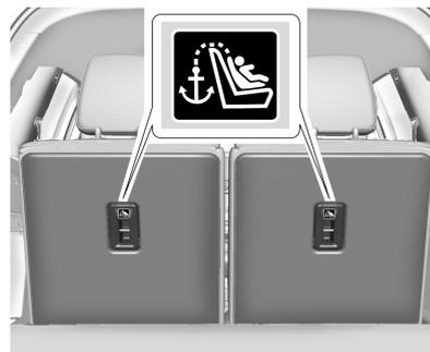
The top tether anchors are on the rear of the seatback for each seating position in the third row.
