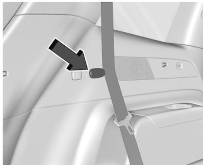
1. Slide the seat belt into the clip on the side of the vehicle. Do this for both sides.
