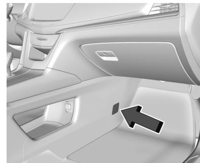
The instrument panel fuse block is in the center console between the driver and passenger seats. To access the fuses, open the fuse panel door, or remove the panel from the passenger side by pulling it out, or see your dealer.
