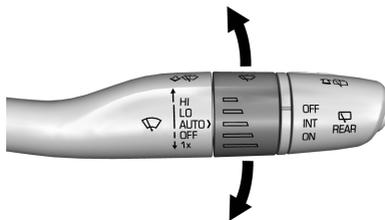
**AUTO** : Use this setting for intermittent wipes when Rainsense is disabled, or Rainsense wipes when Rainsense is enabled. For intermittent
