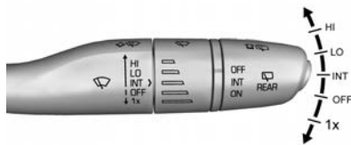
Windshield Wiper without Rainsense (INT Shown)
