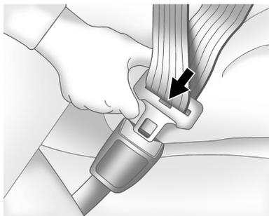
3. Push the latch plate into the buckle until it clicks. Pull up on the latch plate to make sure it is secure. Position the release button on the buckle so that the seat belt could be quickly unbuckled if necessary.
