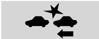
This indicator will display when Automatic Emergency Braking or Front Pedestrian Braking has been turned off or is currently unavailable due to malfunction.
