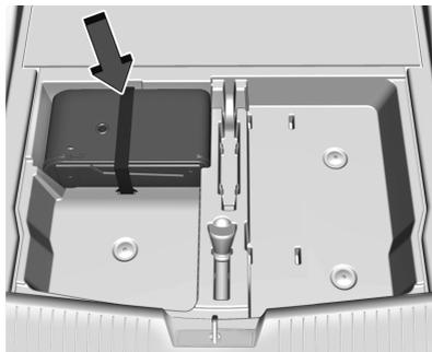
3. Remove the tire sealant and compressor kit bag.
