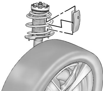
Due to low ramp angles on the V-Series Blackwing, use care when loading the vehicle onto a flatbed carrier. Front spring spacers were provided for lifting the front suspension if more clearance is necessary when towing.
