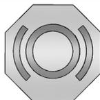
The brake master cylinder reservoir is filled with GM approved DOT 4 brake fluid as indicated on the reservoir cap. See *Engine Compartment Overview* ⇨ 286 for the location of the reservoir.
