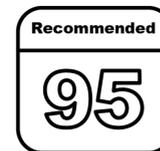
Unleaded petrol with a posted octane rating of 95 RON or greater and with ethanol up to 10% by volume is recommended. If unavailable, unleaded petrol rated at 91 RON can be used, but will result in reduced performance and driveability, and an audible knocking noise may be heard. Once available, 95 RON petrol or
