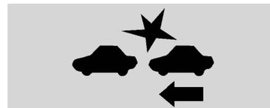
If ACC is engaged, driver action may be required when ACC cannot apply sufficient braking because of approaching a vehicle too rapidly.
