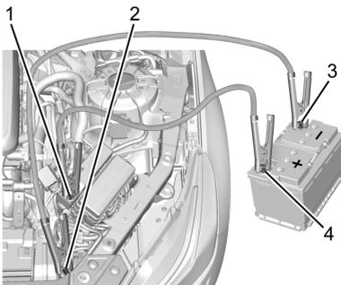
1. Discharged Battery Remote Positive Terminal
