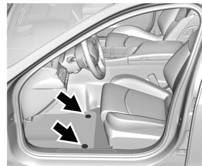
1. Pull up on the rear of the floor mat to unlock the retainers and remove.
