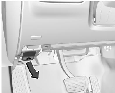
1. Pull the hood release lever with the
