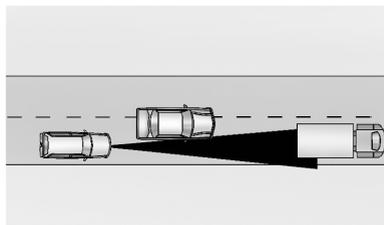
ACC will not detect a vehicle ahead until it is completely in the lane. The brakes may need to be manually applied.
