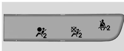
When the vehicle is started, the passenger airbag status indicator will light the symbols for on and off for several seconds as a system check. Then, after several more seconds, the status indicator will light either the on or off symbol to let you know the status of the front outboard passenger frontal airbag and knee airbag.
