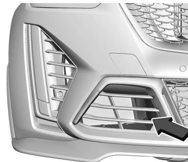
3. Front Brake Cooling Duct
