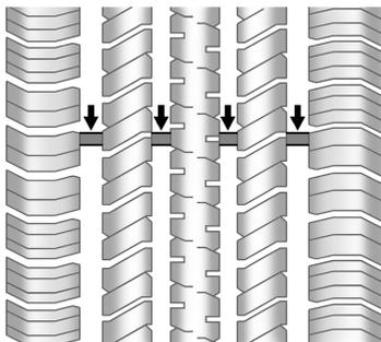
Treadwear indicators are one way to tell when it is time for new tires. Treadwear indicators appear when the tires have only 1.6 mm (1/16 in) or less of tread remaining. See *Tire Inspection* ⇨ 330 and *Tire Rotation* ⇨ 330 for additional information.
