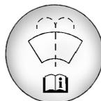
Open the cap with the washer symbol on it. Add washer fluid until the tank is full. See *Engine Compartment Overview* ⇨ 286 for reservoir location.
