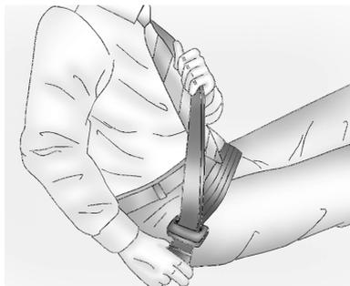
5. To make the lap part tight, pull up on the shoulder belt. It may be necessary to pull the webbing firmly, through the adjustable stop, or move the adjustable stop along the webbing toward the outboard floor anchor, to fully tighten the lap belt across the lap.
