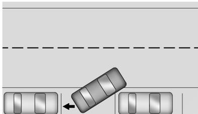
APA will instruct the vehicle to stop once a large enough space is found. Follow the displayed instructions. When instructed to drive in reverse, shift to R (Reverse) to engage automatic steering. The steering wheel will vibrate briefly as a reminder to remove hands from the steering wheel. Check surroundings and continue braking or accelerating as
