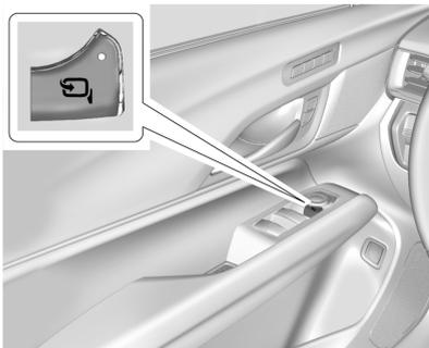
If equipped, press
