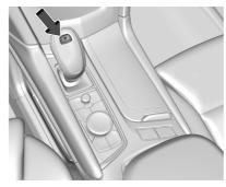
**P** : This position locks the drive wheels. Use P (Park) when starting the vehicle to prevent the vehicle from moving easily.
