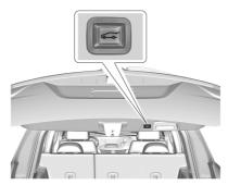
Press any liftgate button, the touch pad, or  $\overline{32}$  on the remote key while the liftgate is moving to stop it. Pressing any liftgate button or pressing  $\overline{32}$  twice quickly on the remote key again restarts the operation in the reverse direction. Pressing the touch pad on the liftgate handle will restart the motion, but only in the opening direction.
