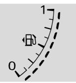
When the ignition is on, the fuel gauge indicates the approximate amount of fuel left in the tank.
