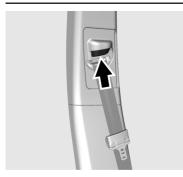
Press and hold the release button while raising or lowering the height adjuster to the desired position.
