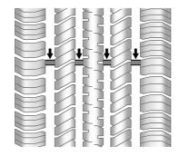
Treadwear indicators are one way to tell when it is time for new tires. Treadwear indicators appear when the tires have only 1.6 mm (1/16 in) or less of tread remaining. See *Tire Inspection*  $\Rightarrow$  287 and *Tire Rotation*  $\Rightarrow$  287.
