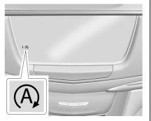
The automatic engine Stop/Start feature can be disabled and enabled by touching the A symbol on the center stack. Auto Stop is enabled each time you start the vehicle.
