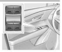
The power windows work when the ignition is on, in accessory mode, or when Retained Accessory Power (RAP) is active. See Retained Accessory Power (RAP)  $\Rightarrow$  191.
