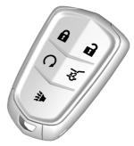
• Press to lock all doors and the fuel door. The turn signal indicators may flash and/or the horn may sound on the second press to indicate locking. To view available settings for this feature, touch the Settings icon on the infotainment home page. Select "Vehicle" to display the list of available options and select "Remote Lock, Unlock, Start".
