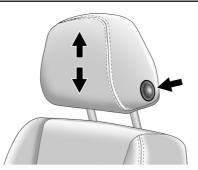
The height of the head restraint can be adjusted.
