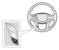
If equipped with a heated steering wheel, press to turn on or off. An indicator light next to the button is lit when the feature is turned on.
