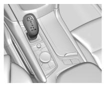
The shift pattern is displayed in the top of the shift lever. The selected gear position will illuminate red on the shift lever, while all others will be displayed in white. If the
