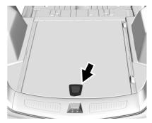
Pull up on the handle to lift the load floor. Use the hook to hold the load floor open. See *Rear Storage* ⇔ 79.
