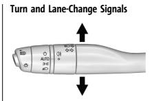
Move the lever all the way up or down to signal a turn.
