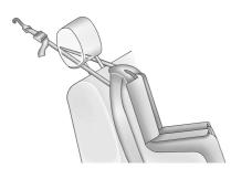
If the position you are using has an adjustable headrest or head restraint, adjust it accordingly to allow proper fitment. If you are using a dual tether, route the tether around the headrest or head restraint posts.
