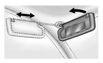
Pull the sun visor down to block glare. Detach the sun visor from the center mount to pivot to the side window and, if equipped, extend along the rod.
