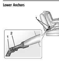
Lower anchors (1) are metal bars built into the vehicle. There are two lower anchors for each LATCH seating position that will accommodate a child restraint with lower attachments (2). Top Tether Anchor
