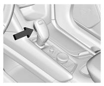
This vehicle is equipped with an electronically controlled transmission. The shift lock release button is designed to prevent inadvertent shifting out of P (Park) unless the vehicle is on, the brake pedal is applied, and the shift lock release button is pressed.
