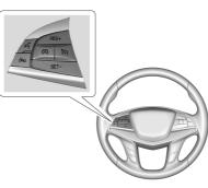
(S) : Press to turn the system on and off. A white indicator appears in the instrument cluster when cruise is turned on.
