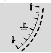
This gauge measures the engine coolant temperature.
