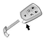
To remove the key, press the button on the side of the remote key, near the bottom, and pull the key out. Never pull the key out without pressing the button.
