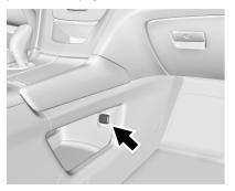
The vehicle has two accessory power outlets: one on the lower center floor console and one in the rear cargo area.
