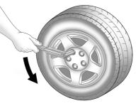
2. Turn the wheel wrench counterclockwise to loosen all the wheel nuts, but do not remove them yet.
