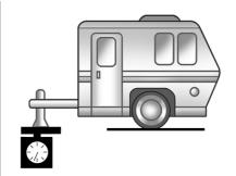
The trailer tongue weight contributes to the Gross Vehicle Weight (GVW). GVW includes the curb weight of your vehicle, any passengers, cargo, equipment, and the trailer tongue weight. Vehicle options, passengers, cargo, and equipment reduce the maximum allowable tongue weight the vehicle can carry, which also reduces the maximum allowable trailer weight.
