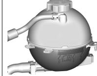
Check to see if coolant is visible in the coolant surge tank. If the coolant inside the coolant surge tank is boiling, do not do anything else until it cools down. If coolant is visible but the coolant level mark is not at or above the indicated mark, add a 50/50 mixture of clean, drinkable water and DEX-COOL coolant. Be sure the cooling system is cool before this is done. See Engine Overheating  $\Rightarrow 263$ .
