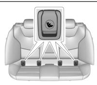
The lower anchors are located under the labeled covers on the seat cushion near the crease between the seatback and the seat cushion.
