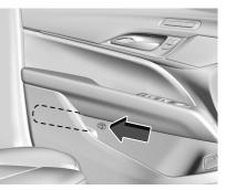
Slide a compact umbrella no larger than 6 cm (2.36 in) in diameter into the opening on the driver or passenger door.
