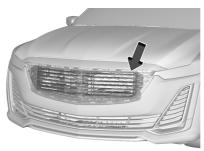
The vehicle may have a shutter system designed to help improve fuel economy. Always keep the shutter system clear of debris, snow and ice. If the check engine light is activated, please check to see if the shutter system is clear of debris, snow or ice.
