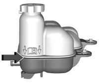
If coolant is visible but the coolant level is not at or above the indicated mark, add a 50/50 mixture of clean drinkable water and DEX-COOL coolant.
