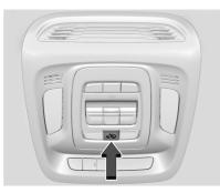
It is recommended that the intrusion and inclination sensor be deactivated if pets are left in the vehicle or the vehicle is being transported. With the vehicle turned off, press in the front overhead console. The indicator light will come on
