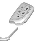
Press the button on the side of the remote key and pull the mechanical key out. Never pull the mechanical key out without pressing the button.
