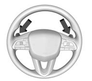
If equipped, vehicles with Tap Shift have controls on the back of the steering wheel to manually shift the automatic transmission.
