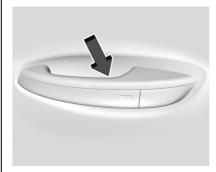
The remote key must be within 1 m (3 ft) of the trunk or door being opened or locked. To unlock and unlatch any door, press the release button on the inside grip area of the outside door handle. Touch the sensor on the front outside door handle to lock. See "Keyless Access Operation" in *Remote Key Operation*  $\Rightarrow$  7.
