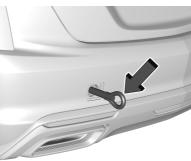
If equipped, carefully open the cover by using the small notch that conceals the rear tow eye socket. Install the tow eye into the socket and turn it until it is fully tightened. When the tow eye is removed, reinstall the cover with the notch in the original position.
