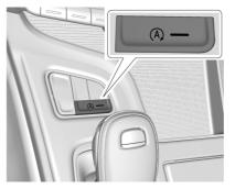
The automatic engine Stop/Start feature can be disabled and enabled by pressing  $\bigcirc$ . Auto Stop/Start is enabled each time you start the vehicle. When the  $\bigotimes$  indicator is illuminated, the system is enabled.
