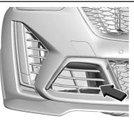
3. Front Brake Cooling Duct
