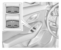
Power windows work when the ignition is on, in accessory mode, or when Retained Accessory Power (RAP) is active. See Retained Accessory Power (RAP)  $\Rightarrow$  202.
