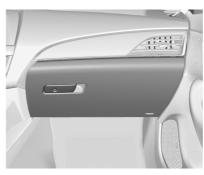
Pull the handle from the side to open the glove box. Close until it latches. Use the vehicle key to lock or unlock.
