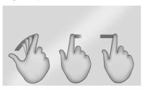
Fling or swipe is used to scroll through a list, pan the map, or change page views. Do this by placing a finger on the display then moving it rapidly up and down or right and left.
