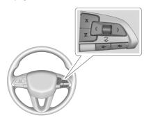
Press  $\leq$  or > to access the cluster applications. Use the thumbwheel to scroll  $\land$  or  $\lor$  through the list of available features. Press the thumbwheel to select. Not all applications will be available on all vehicles.  Info Tiles Selection/Trip Computer/ Maintenance/Driver Assistance: The selected Driver Information Center (DIC) displays can be viewed. See Driver Information Center (DIC) (Base Level)
