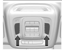
Press the lamp lenses to manually turn on or off the front reading lamps.
