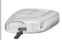
2. Use the mechanical key blade in the slot to remove the battery cover by hand.
