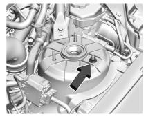
4. Loosen the final strut top mount fastener. Do not completely remove this fastener.
