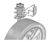
Due to low ramp angles on the V-Series Blackwing, use care when loading the vehicle onto a flatbed carrier. Front spring spacers were provided for lifting the front suspension if more clearance is necessary when towing.
