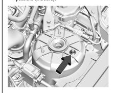
With the suspension located as far inboard as possible, retighten the loose fastener and torque it to 22 N•m (194 lb in).
