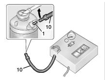
4. Attach the air only hose (10) to the sealant canister inlet valve (1) by turning it clockwise until tight.
