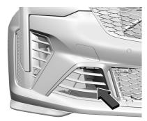
2. Front Brake Cooling Duct
