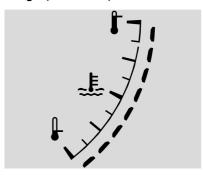
This gauge measures the temperature of the vehicle's engine.
