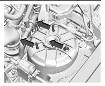
Reposition the suspension/strut assembly so that the strut top mount is located as close to the center of the vehicle as possible (inboard).
