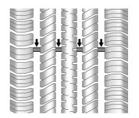
Treadwear indicators are one way to tell when it is time for new tires. Treadwear indicators appear when the tires have only 1.6 mm (1/16 in) or less of tread remaining. See *Tire Inspection* ⇔ 292 and *Tire Rotation* ⇔ 292.
