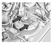
Using a punch, tap out the strut top mount alignment pins. Use compressed air or other method to ensure no debris remains between the top mount and upper spring seat.
