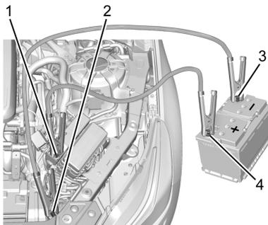
1. Discharged Battery Remote Positive Terminal
