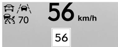
**Speed View :** This displays digital speed in English or metric units, speed limit, vehicle ahead indicator, Lane Departure Warning/Lane Keep Assist, and Adaptive Cruise Control and set speed. Some information only appears on vehicles that have these features, and when they are active.
