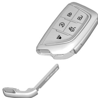
The key inside the remote key is used for the driver door and glove box.
