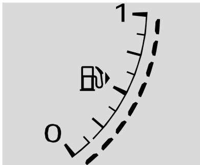
When the ignition is on, the fuel gauge indicates about how much fuel is left in the tank.
