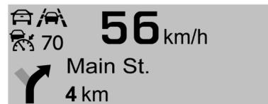
**Navigation View :** This displays digital speed, indicators from speed view along with Turn-by-Turn Navigation information, vehicle ahead indicator, Lane Departure Warning/Lane Keep Assist, Adaptive Cruise Control, and set speed in some vehicles. The compass heading is displayed when navigation routing is not active.
