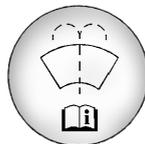
Open the cap with the washer symbol on it. Add washer fluid until the tank is full. See *Engine Compartment Overview* ⇨ 271 for reservoir location.
