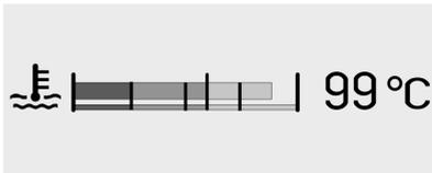
This gauge shows the engine coolant temperature.
