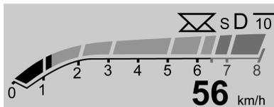
**Performance View :** This displays digital speed, indicators from speed view along with rpm reading, transmission positions, Shift Timing Light Position (V-Series only), and gear shift indicator.
