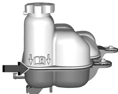
1. With a cold system, add coolant to the indicated line on the surge tank.
