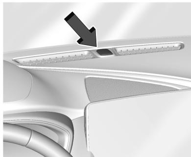
If equipped, the light sensor is on top of the instrument panel or on the windshield near the rearview mirror. Do not cover the sensor, otherwise the headlamps will come on when they are not needed.
