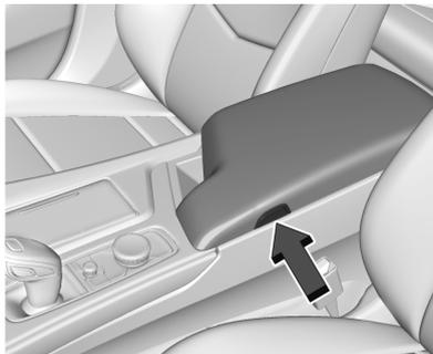
Press the button and lift to access the storage area. There is an accessory power outlet, two USB ports, and an SD card slot inside. See *Power Outlets* ⇨ 89 or *USB Port* ⇨ 146.
