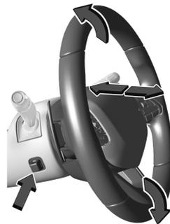
If equipped, the control is on the left side of the steering column.
