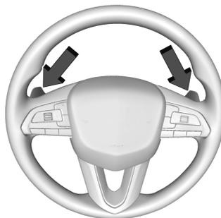
If equipped, vehicles with Tap Shift have controls on the back of the steering wheel to manually shift the automatic transmission.
