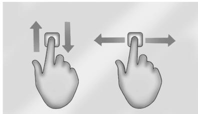
Drag is used to move applications on the Home Page, or to pan the map. To drag the item, it must be held and moved along the display to the new location. This can be done up, down, right, or left. This feature is only available when vehicle is parked and not in motion.
