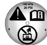
1. Remove the coolant surge tank pressure cap when the cooling system, including the coolant surge tank pressure cap and upper radiator hose, is no longer hot. Turn the pressure cap slowly counterclockwise. If you hear a hiss, wait for that to stop. This will allow any pressure still left to be vented out the discharge hose.
