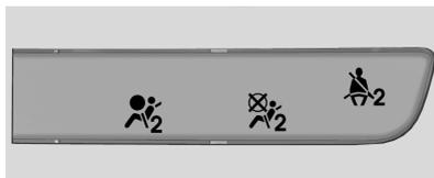
The symbols for on and off will be visible during the system check. When the system check is complete, either the symbol for on or off will be visible. See *Passenger Airbag Status Indicator* ⇨ 102.
