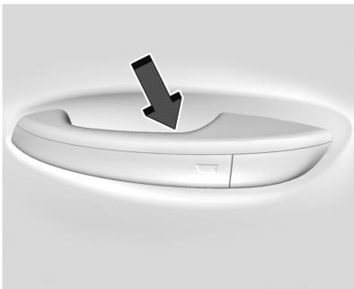
The remote key must be within 1 m (3 ft) of the trunk or door being opened or locked. To unlock and unlatch any door, press the release button on the inside grip area of the outside door handle. Touch the sensor on the front outside door handle to
