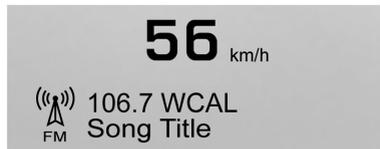
**Audio/Phone View :** This displays digital speed, indicators from speed view along with audio/phone information, vehicle ahead indicator, Lane Departure Warning/Lane Keep Assist, Adaptive Cruise Control, and
