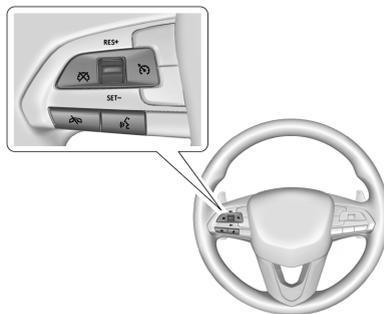
**Ⓢ** : Press to turn the system on and off. A white indicator appears in the instrument cluster when cruise is turned on.
