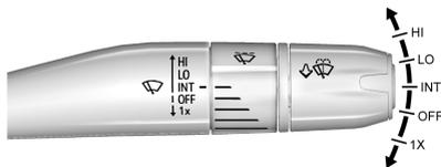
With the ignition on or in ACC/ACCESSORY, move the windshield wiper lever to select the wiper speed.
