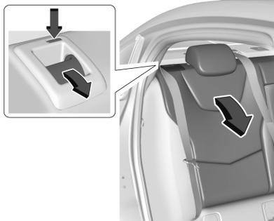
2. Pull the lever on top of the seatback toward you to unlock the seatback.
