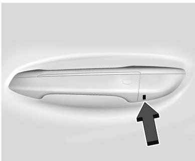
1. Insert the mechanical key into the slot at the bottom of the handle and push upward all the way until the cover frees. Do not pry or pull on the key.
