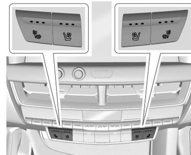
If equipped, the buttons are near the climate controls on the center stack. To operate, the engine must be running.
