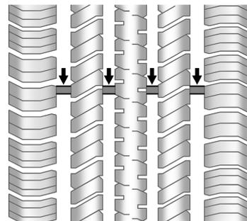
Treadwear indicators are one way to tell when it is time for new tires. Treadwear indicators appear when the tires have only 1.6 mm (1/16 in) or less of tread remaining. See *Tire Inspection* ⇨ 309 and *Tire Rotation* ⇨ 309 for additional information.
