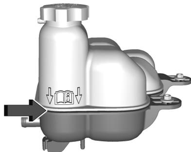
3. Fill the surge tank with the proper mixture to the indicated level mark.
